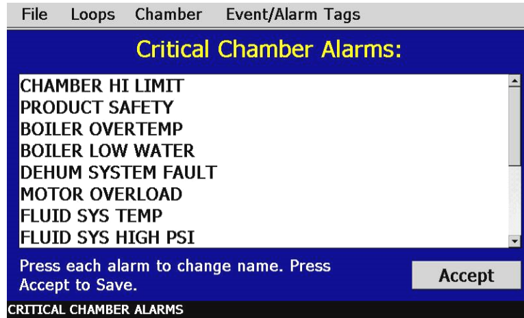
Figure 8-16 Critical Chamber Alarm Names
